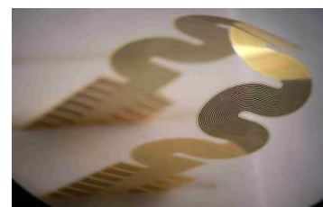
flexible metal paths embedded in polymer
